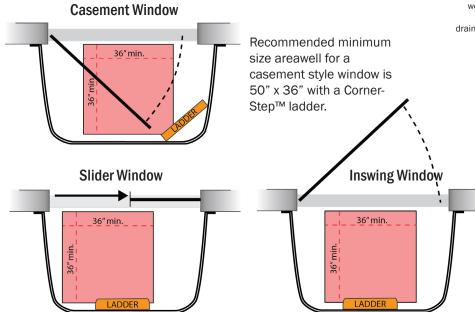
Minimum size window well for both a slider and inswing style window are 42" x 36" with a Life-Step<sup>TM</sup> ladder.
